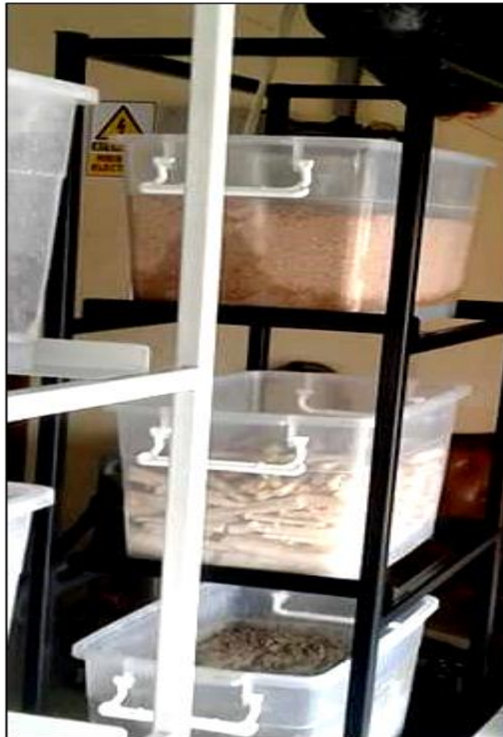
Figure 3. Filtration process. The wastewater is initially discharged from the upper compartment and flows down in contact with the materials into the lower chambers, where the treated liquid is collected at the bottom.
