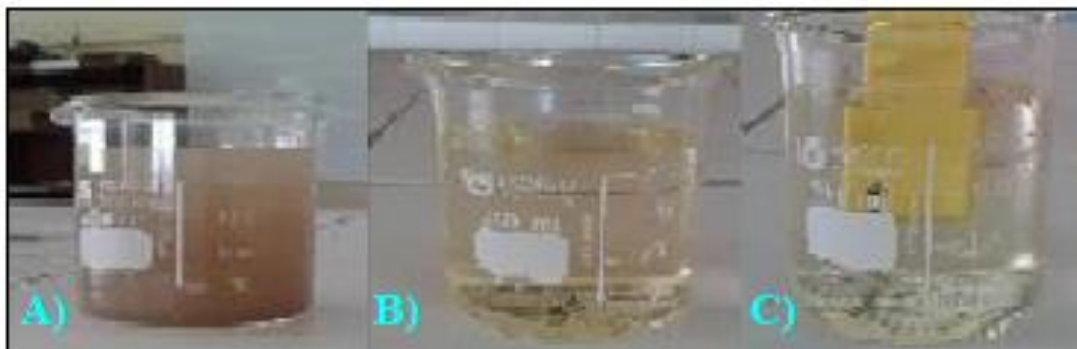
Figure 4. The sequence of wastewater treatment (A → B → C) as it is treated. A gradual decrease in turbidity and suspended solids in the water is evident.
