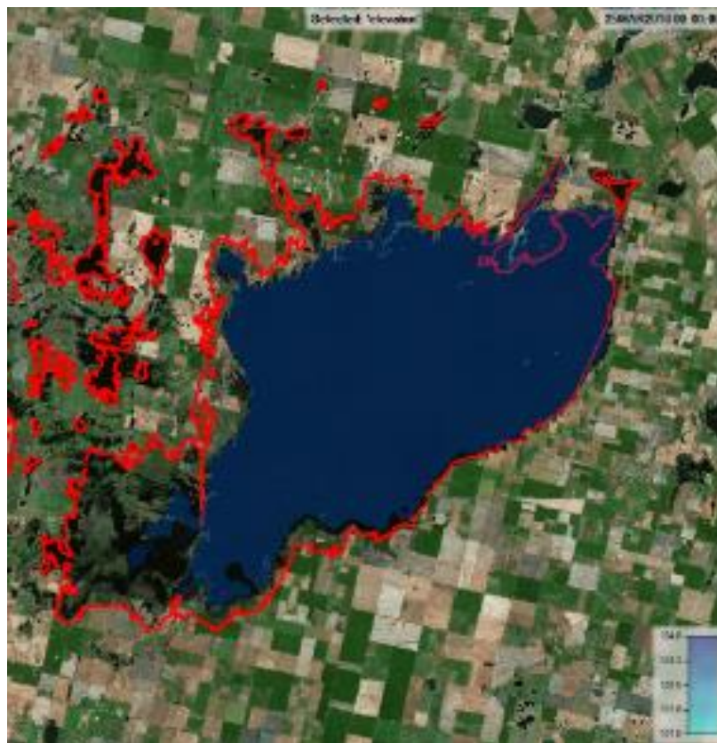
Figure 20. Comparison of the maximum level obtained with HEC-RAS and the maximum flood envelope (defined according to the MNDWI index) for scenario 2.
