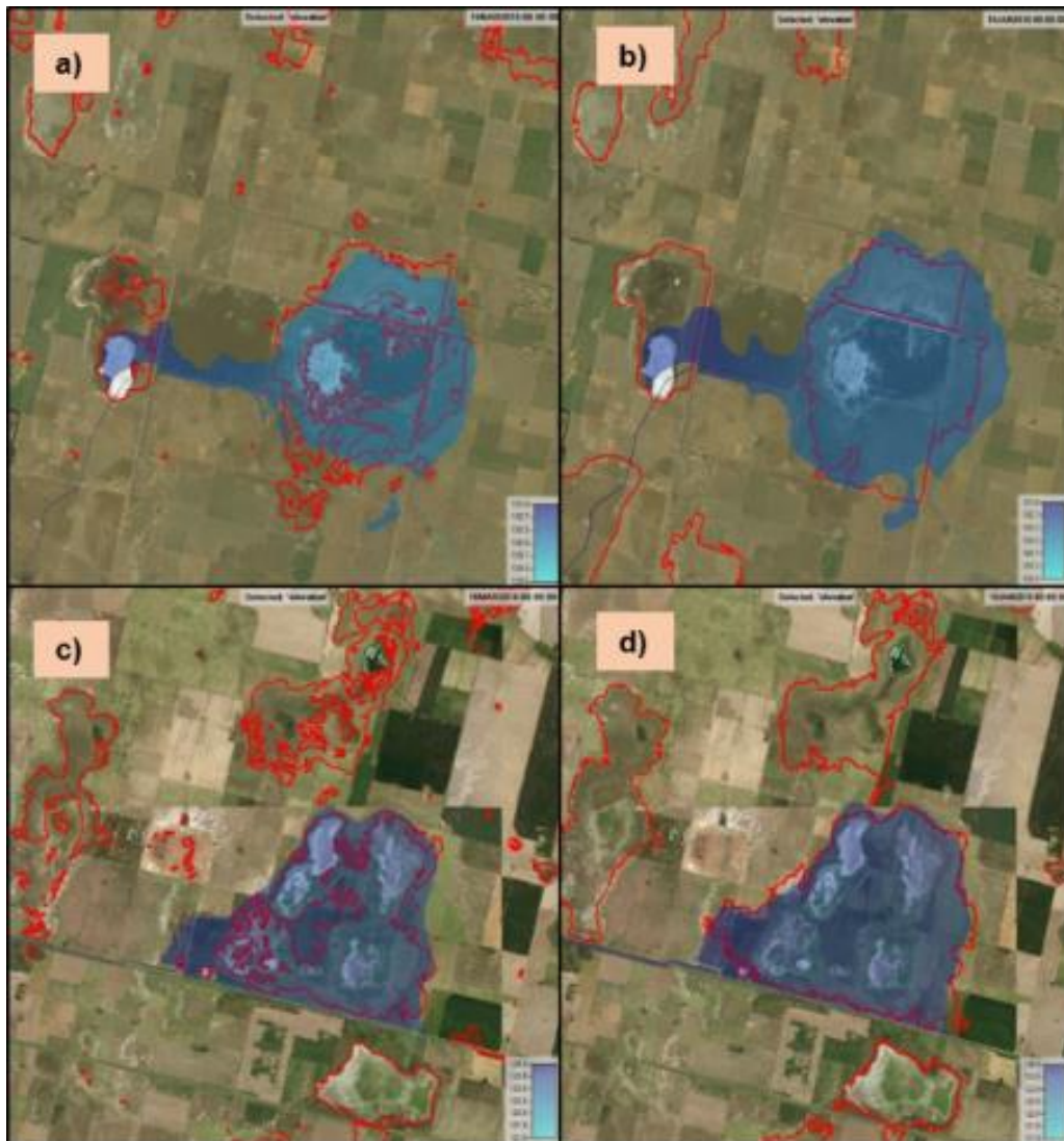
Figure 19. Level results obtained for scenario 4: a) reservoir 2-03/16/2016; b) reservoir 2 for maximum level; c) reservoir 4-03/16/2016; d) reservoir 4 for maximum level.
