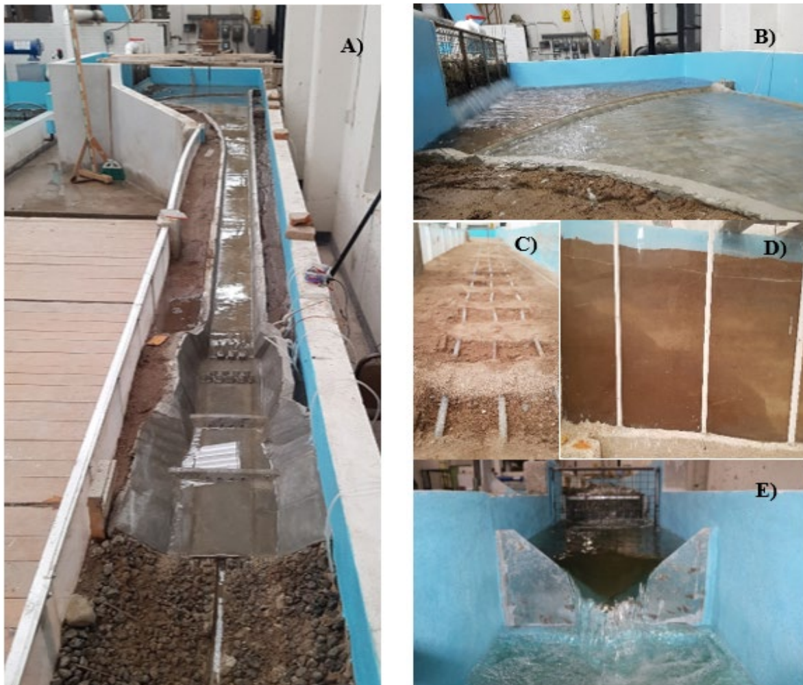
Figure 3. A) Physical model, complete view of the overflow works; B) velocity reducing screen, vessel, crest, initial part of the discharge channel; C) streamlines in the compacted soil profile; D) transverse and longitudinal drains, placed in the lower part of the discharge channel; E) triangular 90° weir.
