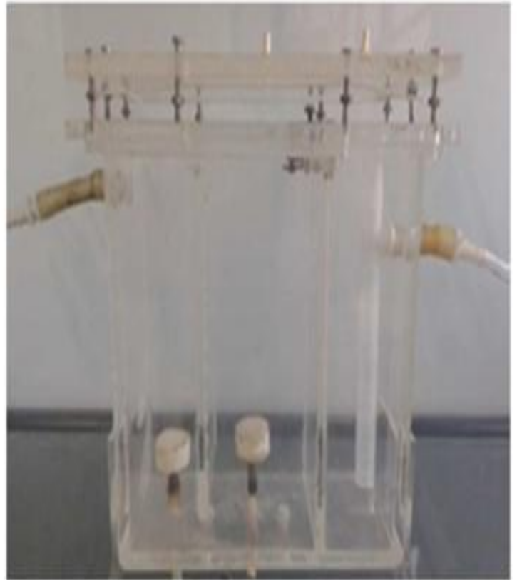
Figure 2. Scheme and picture of the tank for fat trap and primary sedimentation. Zones I, II, and III.
