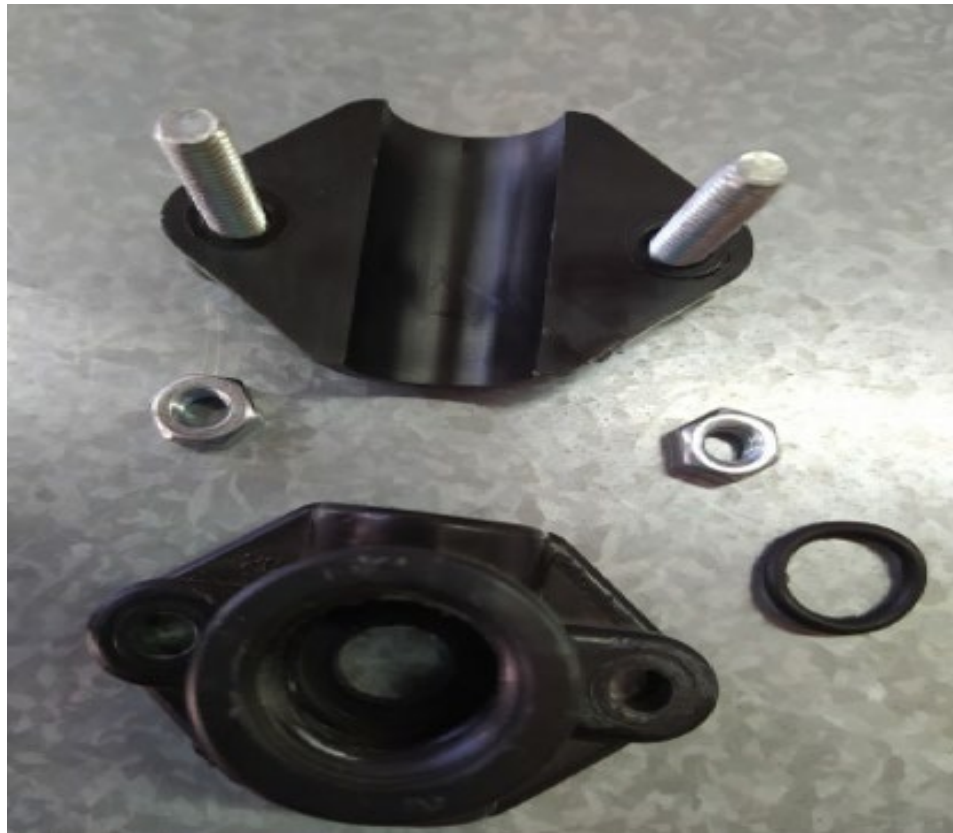
Figure 5. Flexible coupling to attach pressure transducers to hydraulic pipes.
