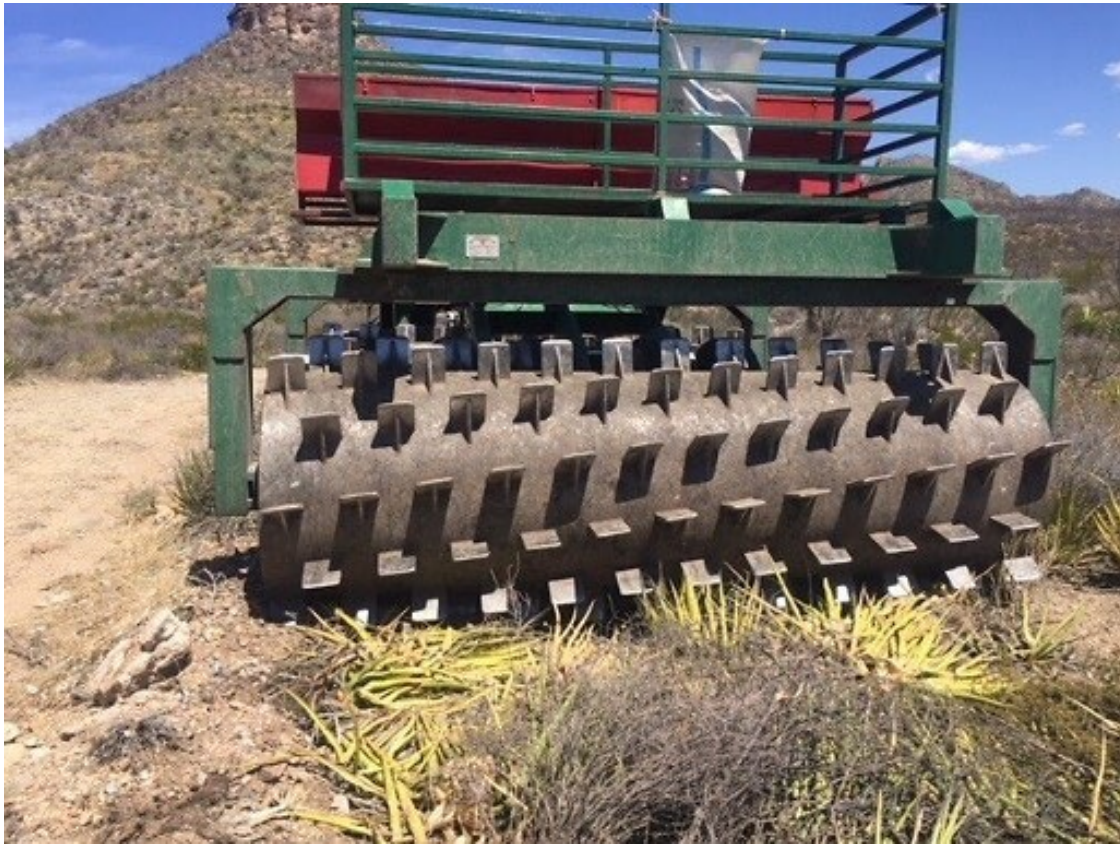
Figure 2. Use of the land imprinter for planting buffel grass in areas of the experimental watershed.
