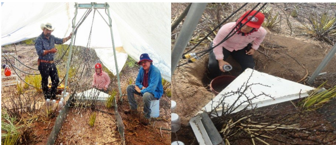
Figure 9. Rainfall simulation and runoff sampling.
