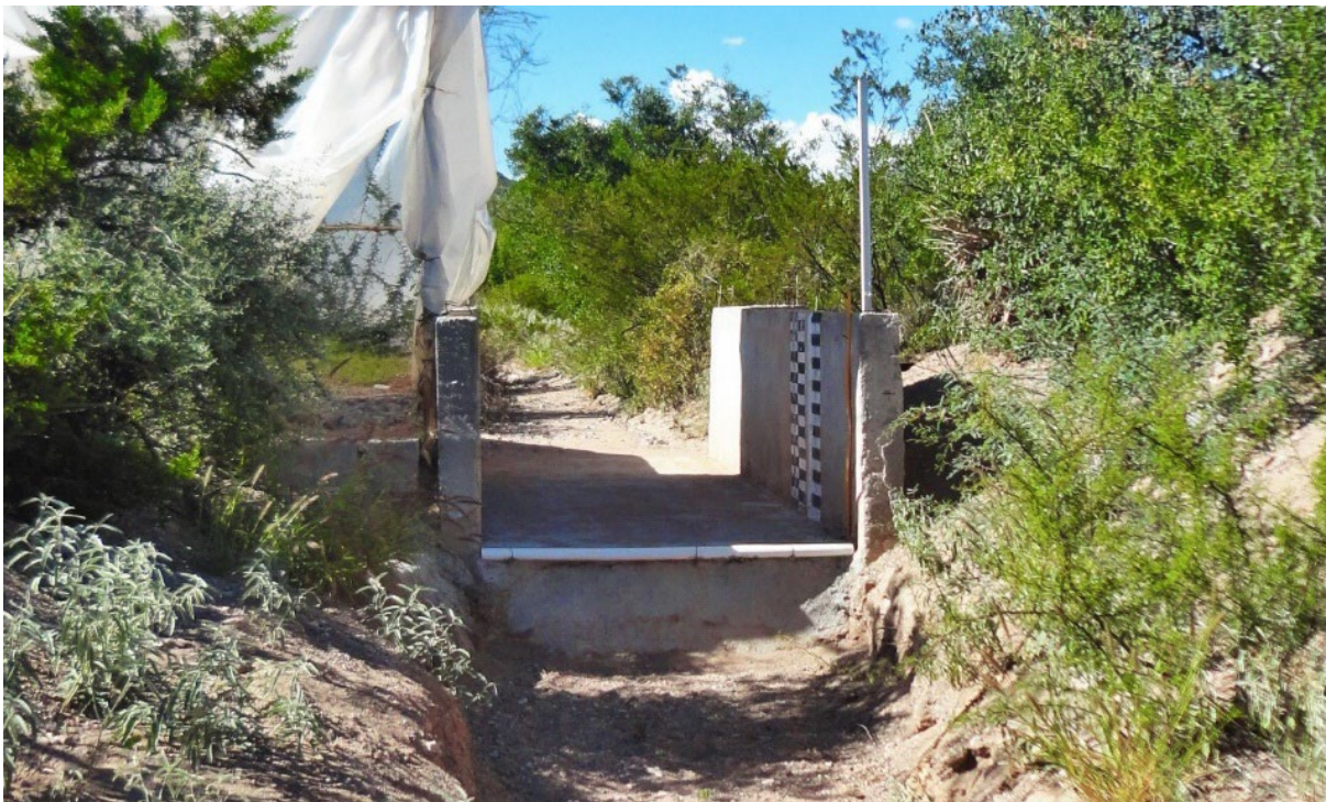
Figure 5. Hydraulic section of the flume at the outlet of the experimental watershed.
