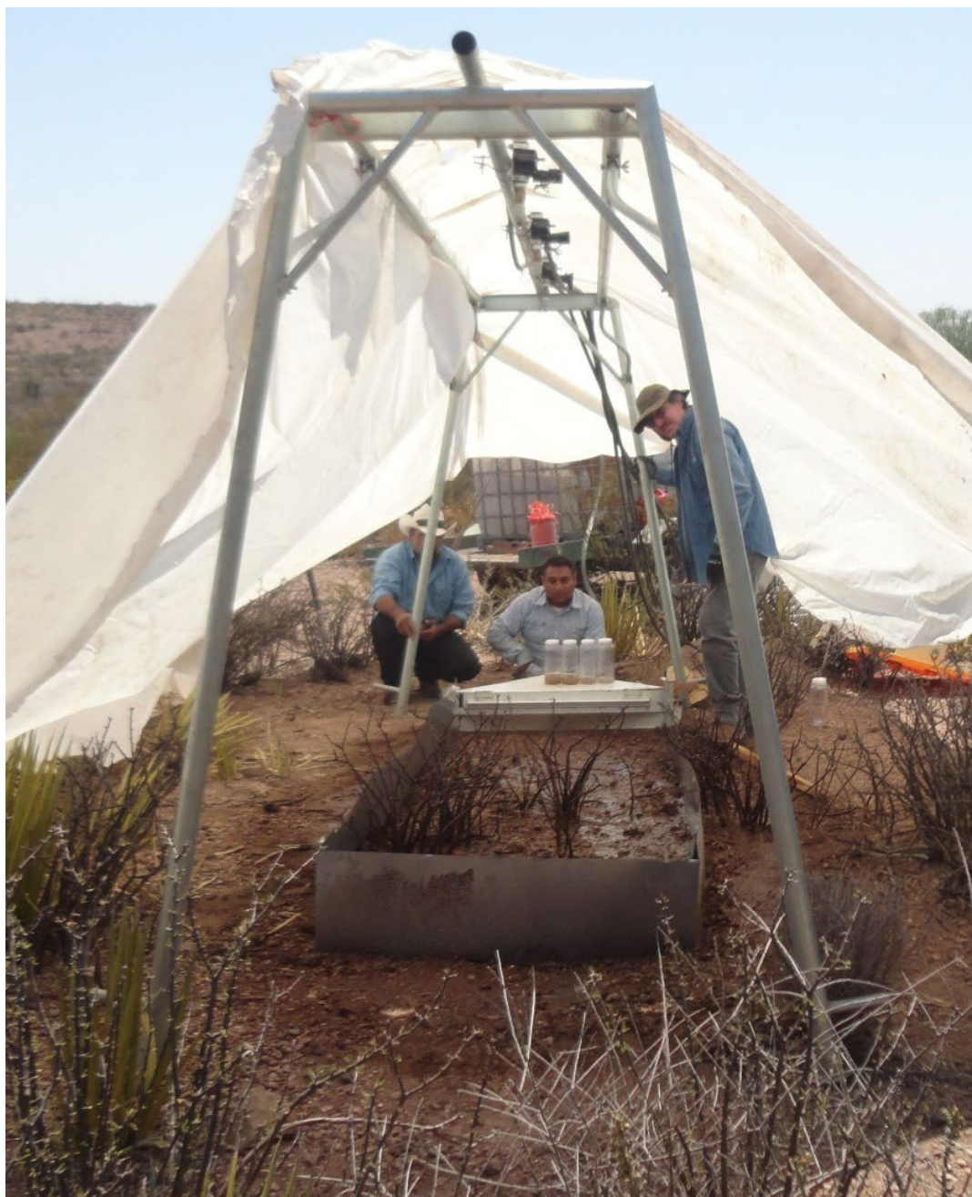
Figure 7. Rainfall simulator in the watershed.
