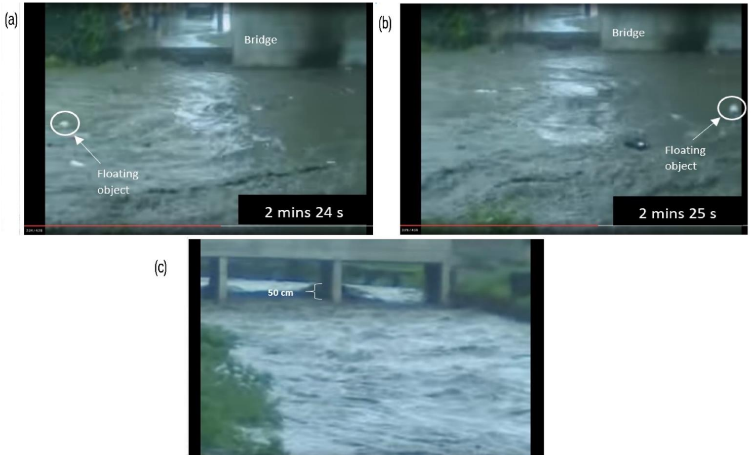
Figure 7. Key images for measurements from YouTube videos: (a) show the extent of the “control section” when a floating object enters, and (b) when it exits the section. The bridge access of the left bank can be observed. One of the HWE points was placed in that location. In (c) the section employed to apply the velocity-head method. Notice the jump in the piers of the smaller bridge (SB) located immediately upstream from the study reach.
