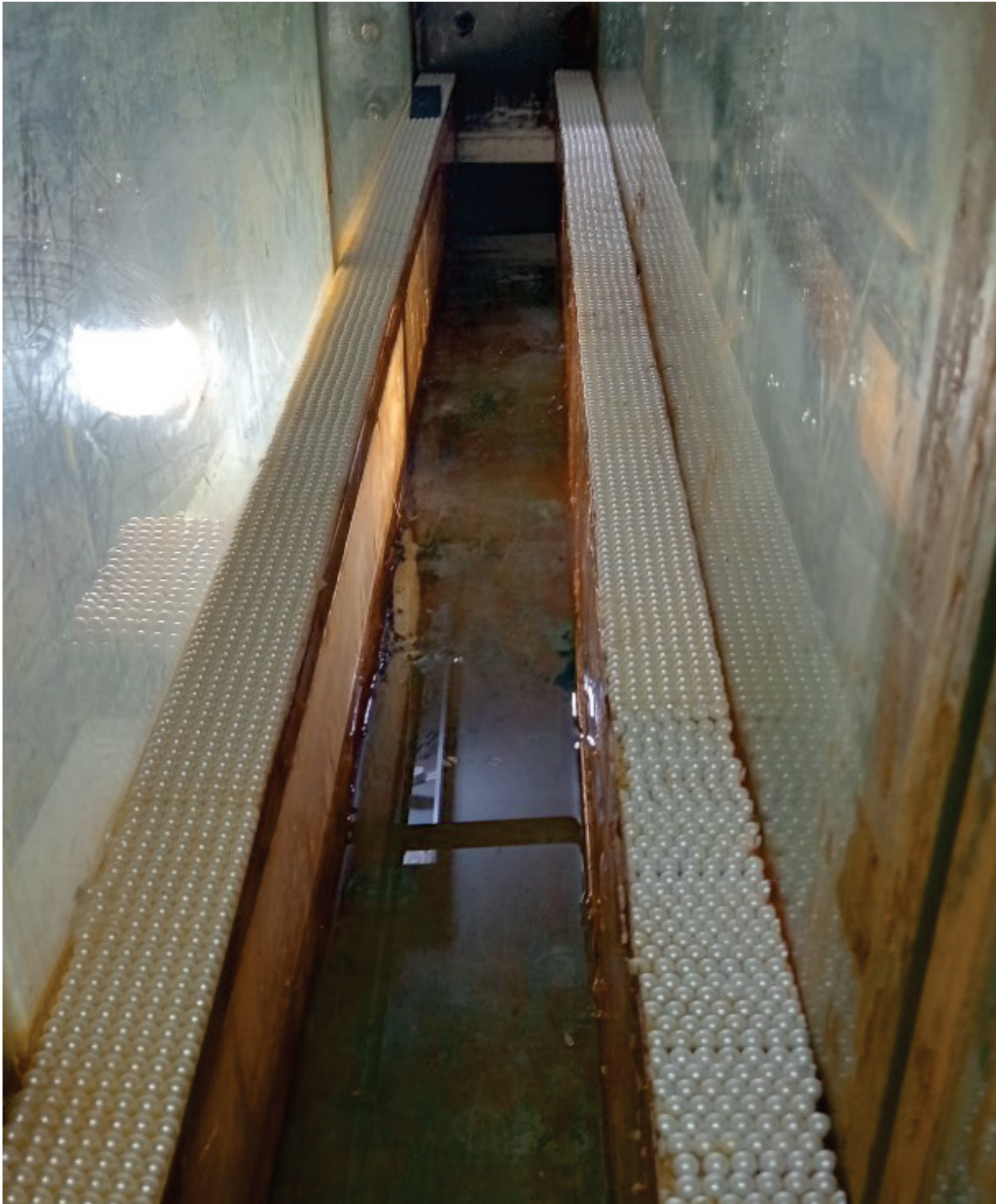
Figure 3. Experimental setup of the compound channel with roughened floodplains (major bed) and a smooth main channel.
