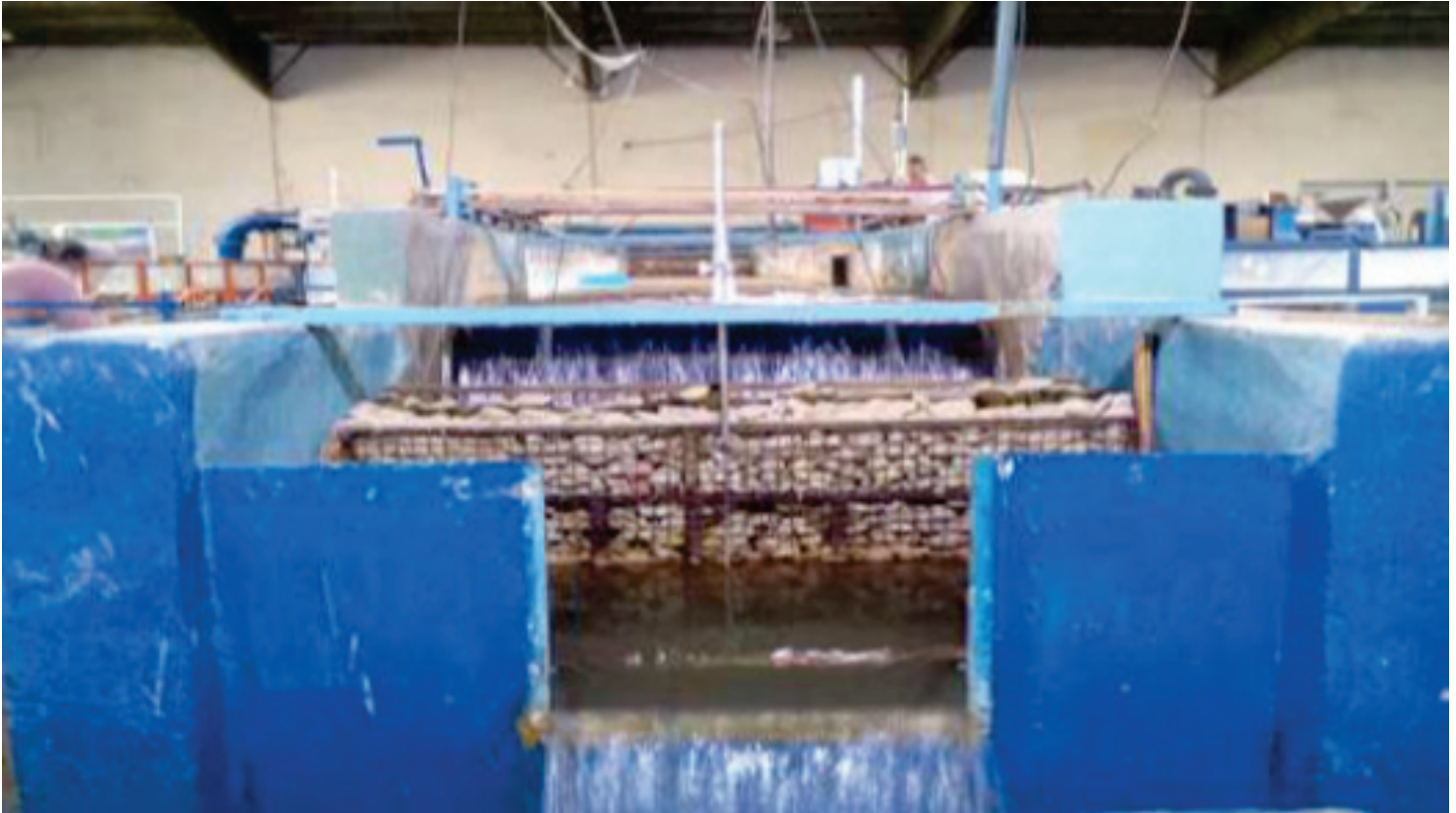
Figure 6. The rectangular weir used in the experimental process.
